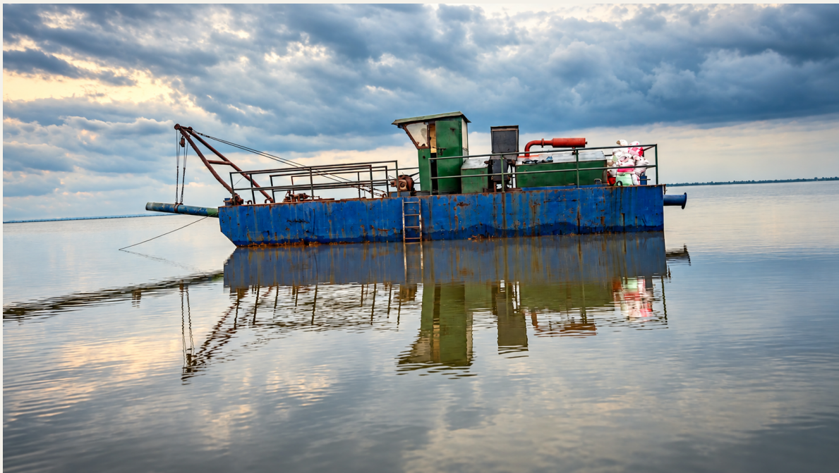
Floating dredging vessel showing the working platform, cabin, lifting equipment and pipework.
