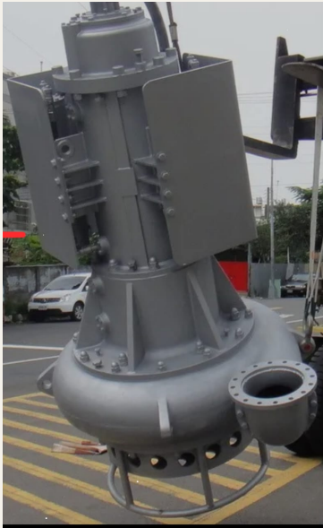
01 Submersible pump body with a vertical motor housing and side discharge flange.
