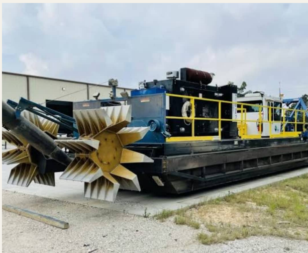
03 Dredger onshore showing the cutter assembly, working platform and machinery.
