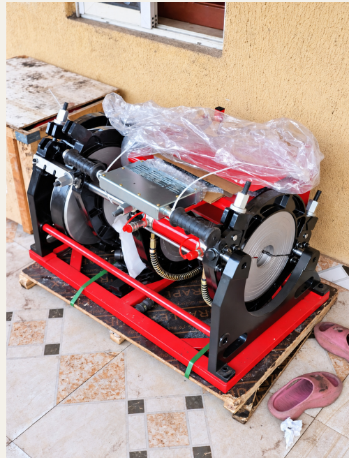
13 Butt-fusion equipment used to prepare HDPE pipe joints.
