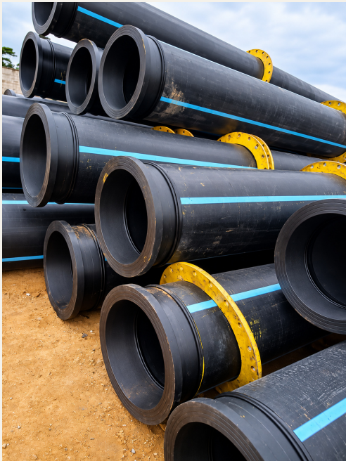
04 Flanged HDPE pipe sections prepared for deployment.
